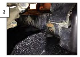
Install the supplied bolts through the rear skid plate mount and into the crash bar, then secure with a locking nut.
