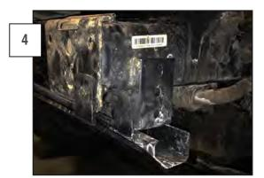
Install the skid plate to the front side of the frame with the stock nut, or use the bolt that holds an aftermarket bumper to the frame.
