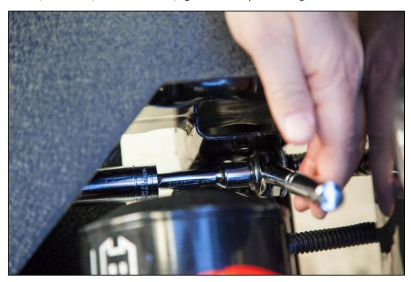
17. Depending on the clearance, you may need to remove the socket extension bar to access the interior bumper mount bolts.
