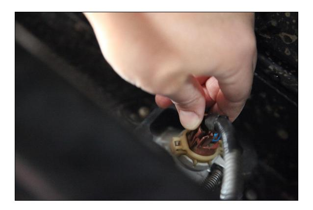
5. Using a combination of some or all of the following: 18 mm deep well socket, socket extension bar, socket swivel attachment, breaker bar, and socket wrench; remove 3 of the 4 front factory bumper mount nuts from each side of the Jeep. Loosen the last nut on each side, but leave in place for safety. Detaching the fog light wiring harness clips may allow for better access to the bumper mount nuts.
