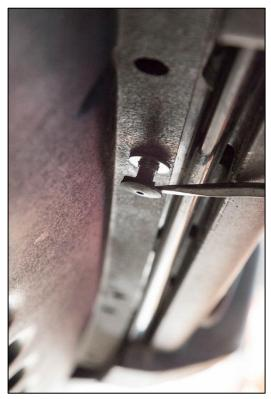
4. Disconnect the factory fog light plugs by depressing the plastic catch and pulling the plug away from the light.
