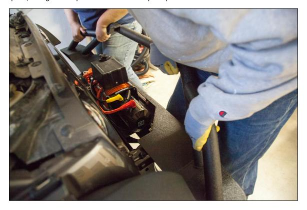
16. Install the provided flat washer, split washer, and nut onto each of the Barricade bumper bolts. Using a combination of some or all of the following: 18 mm deep well socket, socket extension bar, socket swivel attachment, breaker bar, and socket wrench; tighten all 8 bumper mounting nuts.
