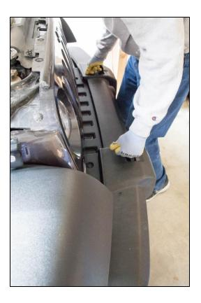
8. Lay Barricade front skid plate in place under front of Jeep, ensuring the bend in the skid plate is aligned directly under the crash bar. Lift the passenger side of the skid plate up into position so the rear mounting tab is directly behind the crash bar. Jack stands may come in handy to help support the skid plate during install.
