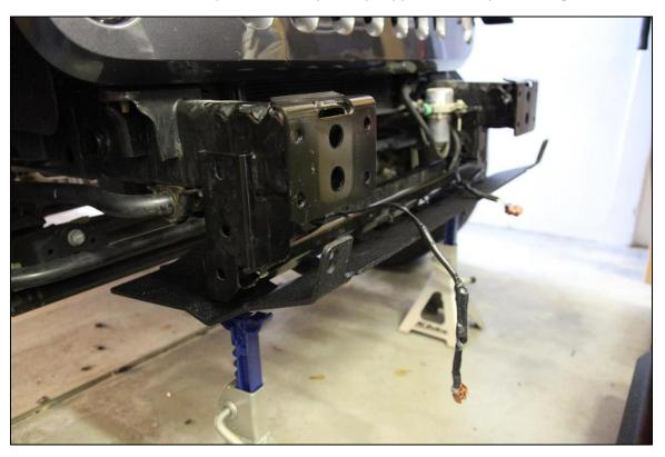
9. Install one flat washer onto one of the provided bolts and insert bolt assembly through skid plate and crash bar mounting holes.
