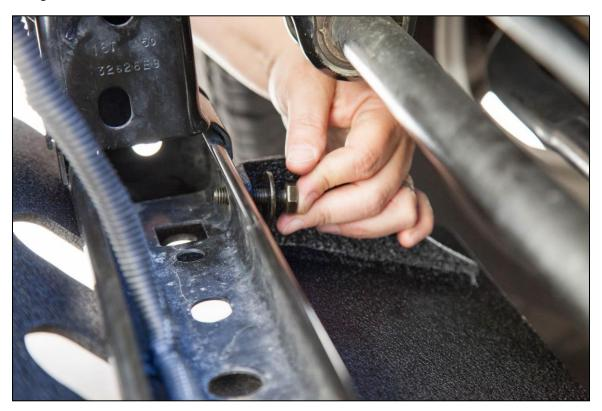
10. Install second flat washer onto bolt protruding into the interior of the crash bar. Install lock nut and make finger tight to keep skid plate in position.
