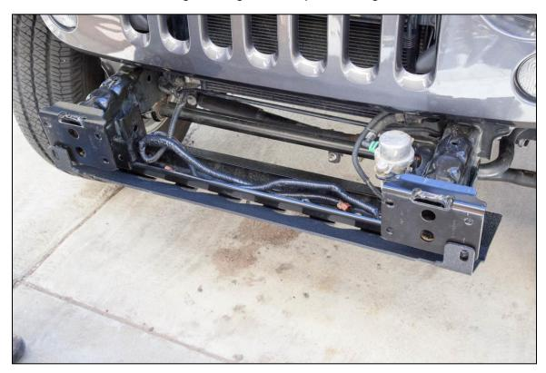
13. *Optional:* Collect the factory spacer plates and install them on the bumper bolts to create more room for your winch, winch cables, and winch cover when your Barricade bumper and winch are installed.
