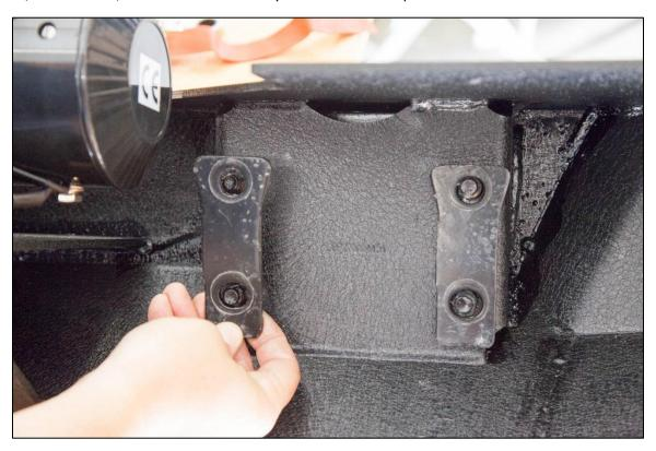
14. Using a 5/8 inch socket or flex head ratcheting wrench and an 11/16 inch socket or flex head ratcheting wrench, tighten the lock nuts on both sides of the skid plate.
