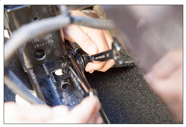
15. If reinstalling a Barricade bumper with a winch, this may be a two-person job because of the weight. Lift bumper into place, sliding the bumper bolts into the factory bumper mount holes.
