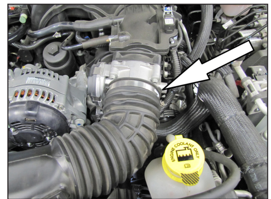
5. Loosen the hose clamp securing the factory intake tube to the throttle body.
