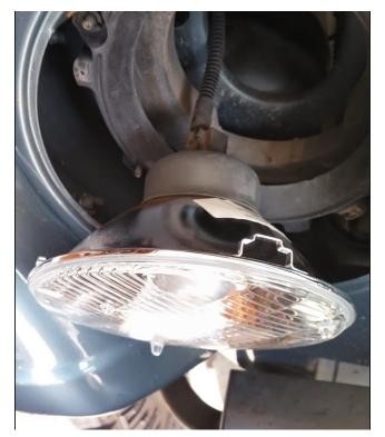
6. Properly seat the Hella headlamp into the headlight socket and while holding in place reinstall the inner housing ring using the four inner ring screws.
