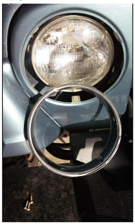
3. Remove the four inner housing screws using the Torx T15 screwdriver or socket. Once the last screw is removed, the inner housing ring will come right out.
