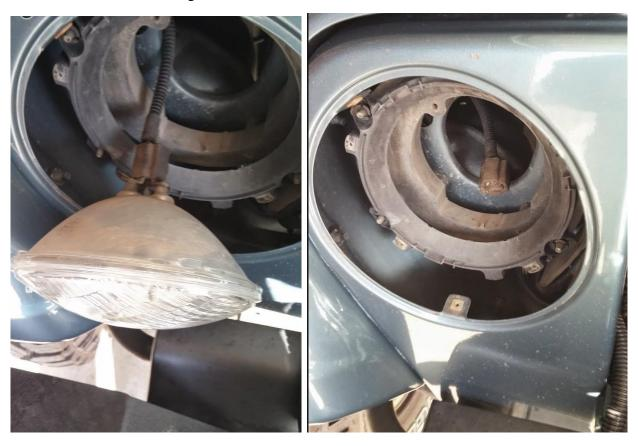
5. Connect the new Hella headlamp into the harness. Turn on the headlights to test the connection before putting everything back together.
