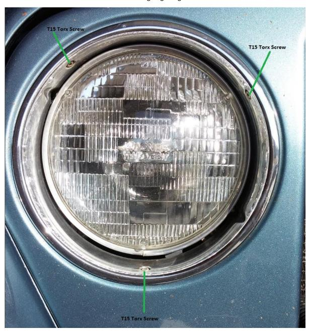
2. Once the screws are removed, gently rotate the outer housing ring counter-clockwise about 1/8" and the ring should pull right out.
