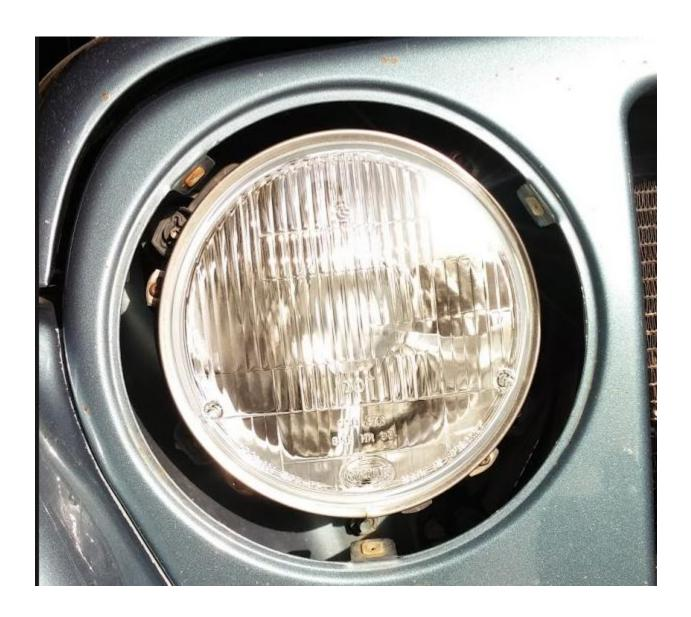
7. Reinstall the outer housing ring with the three outer housing ring screws. First, seat the outer housing ring offset counter-clockwise by approximately 1/8" and once seated, rotate it to the right to line up the holes before installing the screws.
