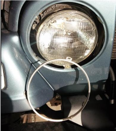
4. You can now easily pull out the old bulb housing and gently disconnect the harness in the back. If your harness has corrosion or is dirty, you may want to clean the connections off to ensure a good connection with the new lights.
