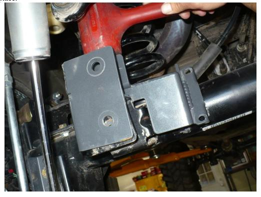
4) Once seated over the axle tube, use an alignment bar to properly line up the bottom
