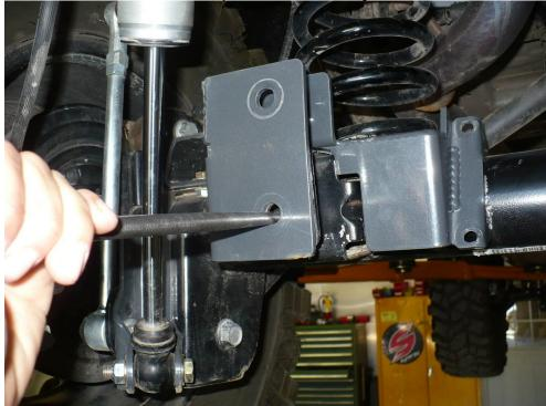
5) Next, install the 1.60" wide spacer provided in the kit in the factory location as shown. Use the 9/16" bolt included in the kit with a washer under the bolt head to
