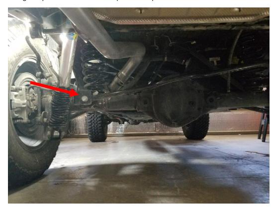
2. Place the new bracket over the original bracket as shown, then use a rubber mallet to tap it down into place until the bolt holes line up. You may also need to use a large screwdriver to further align the bolt holes.
