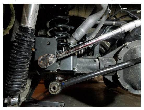
**6.** Now place the track bar in the new bracket and align the holes. The easy way is to have a friend push on the body of the Jeep until they line up. You can also push on the frame while lying under the Jeep. Then insert the stock bolt.
