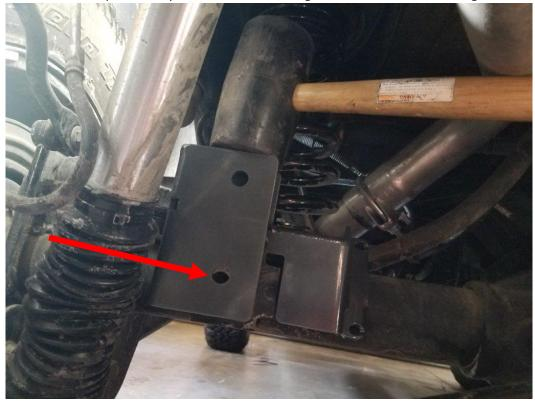
3. Now insert the supplied spacer inside the bracket, then install the supplied bolt with washer as shown. You can use the mallet to tap the bolt all the way through. Then install the supplied washer and nylock nut on the bolt.
