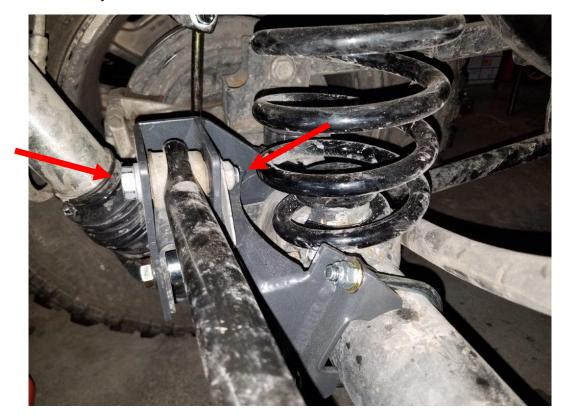
**8.** Synergy recommends using a 2" bumpstop to keep the bracket from hitting the stock exhaust. You can get ones specifically made for this, or you can use hockey pucks. Take 2 hockey pucks, drill a hole through the center, and then install them with a bolt and washer to the axle as shown below. Do this on both driver and passenger sides.
