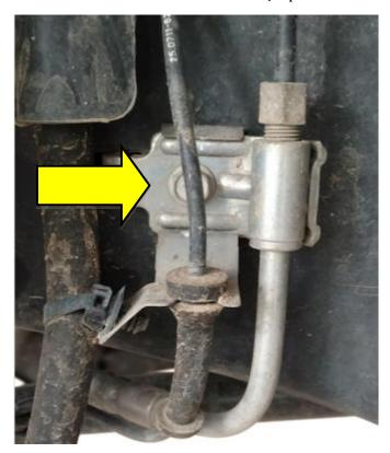
7. Next you will have to remove the ABS bracket. This is the bracket which is located in front of the bottom of the front shock. Locate the bottom bolt of the front shock and you will see the bracket that is holding both the brake line and the ABS line.
