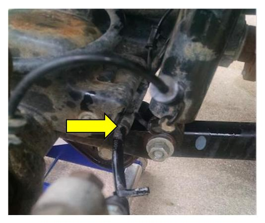
8. To remove the ABS bracket you will first need to remove the bottom shock bolt. Use an 18 mm socket on the bolt head and an 18 mm box wrench on nut. Hold the box wrench to hold the nut still, while using the ratchet to loosen and remove the bolt. Do not lose or discard the bolt as you will need to use it to reconnect the shock!
