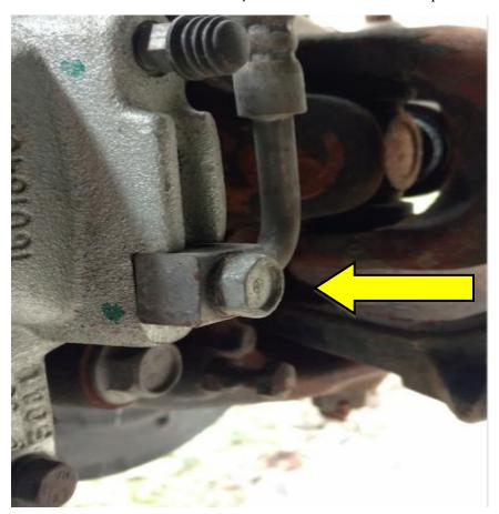
5. Detach the entire ABS line from the brake line, you can do this by opening the rubber clips and then snipping the zip ties. \*\*Be careful not to snip the ABS line when you snip the zip ties.\*\*
