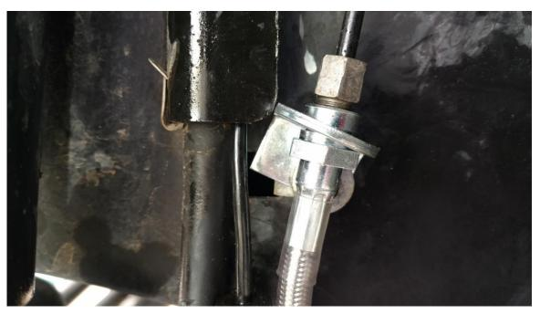
3. Next install the spring clip between the L Mounting Bracket and the top of the Synergy brake line. Line up the clip and then tap it with a rubber mallet to secure it in place.
