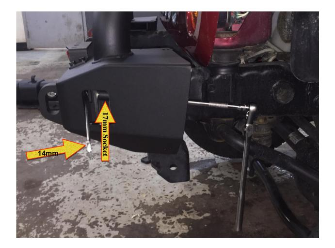
**<u>11.</u>** Tighten the inner two mounting bolts on each side in the same way. Don't forget to use a torque wrench to tighten to 44 Nm
