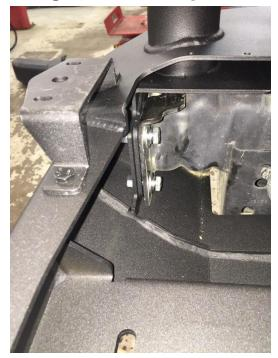
12. (Optional) install running light bracket by placing brackets over mounting holes just inside bull bar of ARB Bumper, and then inserting 13mm bolts and nuts with flat and lock washers on bottom. Tighten with 13mm socket and ratchet. Also torque to 22 Nm.
