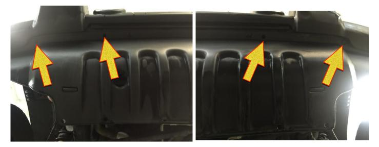
3. Remove two no pressure retaining screws from stock front skid plate hangers with a Phillips head screwdriver or pry bar if you don't plan on reusing the stock hardware. These are located on the back (inside) of the skid plate.
