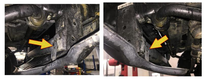
4. Remove the Factory Skid plate.
