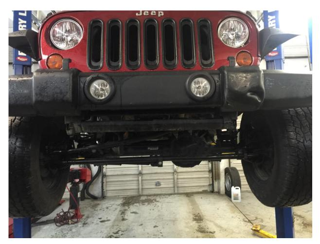
5. With an 18mm Deep socket and 6 inch extension remove the outer two frame horn mounting nuts on the driver and passenger side.
