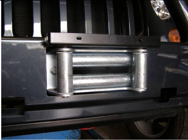
Roller Fairlead installed
