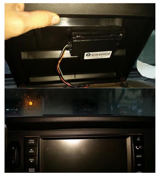
10. Firmly press the panel back end into place
