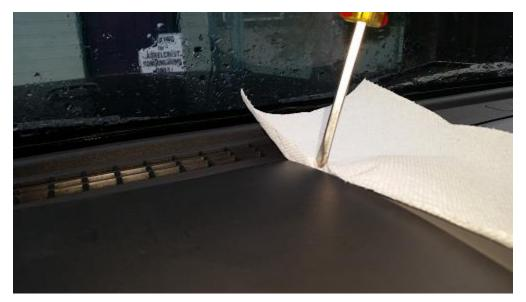
2. Pull the panel towards the interior and then lift the front end up to expose the compass module (this may take some slight jiggling to release the front edge while pulling).
