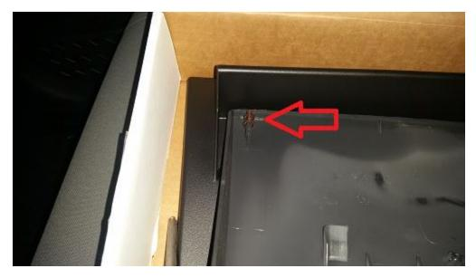
5. Using the flathead screwdriver, remove the clips from the old panel.
