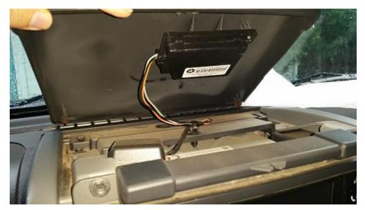
3. Using the Philips head screwdriver, remove the two screws holding the compass unit to the old panel.
