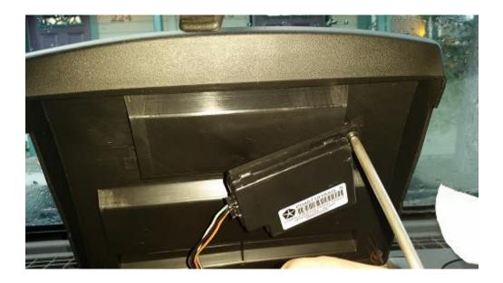
9. Lower the panel into place, sliding the front on first.
