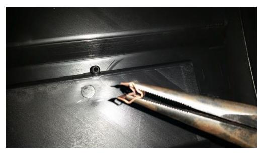
7. Push the clips onto the mounts on the new panel.
