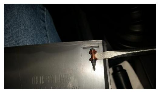
6. Using the needle nose pliers, squeeze the clips back to form for re-use.
