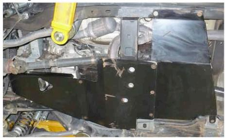
6. You can now install the rear transfer case skid plate, install the skid plate on top of the cross-member skid plate. If you drilled and tapped the gas tank and frame hole to %-20, use the supplied flat head allen bolts, if not us the original bolts, tighten to 35 ft-Ibs.
