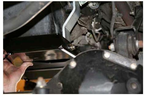
11. Install the passenger side frame brace as shown with the larger hole in the top. Use a W' bolt with a flat washer and flange nut on the top and two 3/8" bolt with a lock nut and flat washer on the bottom.
