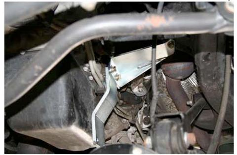
10. Install the front engine skid plate, put the rear on top of the crossmember skid plate and attach the front to the driver side frame brace. Using the W' flat head allen bolts and flange nuts, attach the rear of the engine skid to the front of the crossmember skid. Do not tighten these bolts yet; leave them loose until both of the front brackets are installed.
