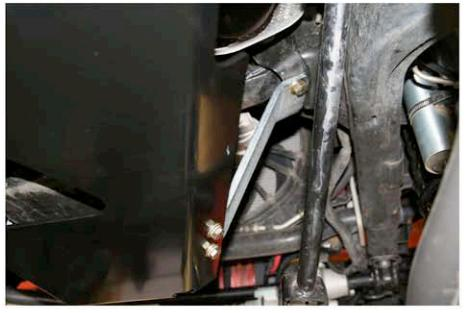
12. Adjust the side to side position of the front engine skid and tighten all the mounting bolts. Tighten the 3/8" bolts to 20 ft-Ibs and the W' bolts to 35 ft-Ibs.
