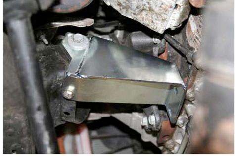
9. Install the driver side frame brace to the frame bracket; the driver side is the shorter of the two. There is no top or bottom and can be installed in either direction. Use the supplied 3/8 bolts, flat
