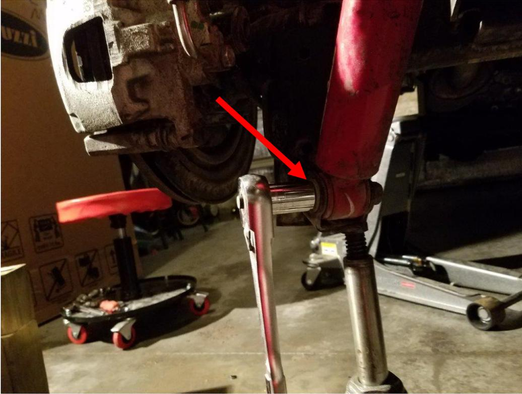
7. Remove the lower plastic clip holding the ABS wire to the frame.
