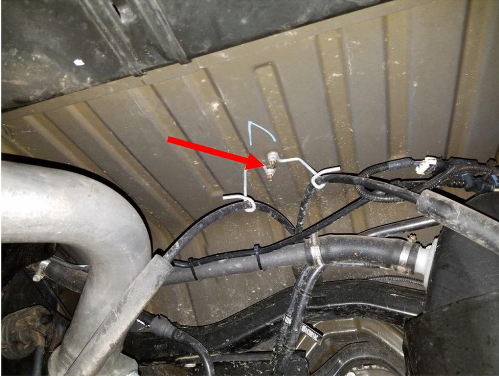
9. Now, using the jack under the axle, slowly lower it until the coil spring is loose. This will require the jack under the frame to be as high as possible. Keep an eye on the brake line and ABS wire, be careful not to overstretch them.
