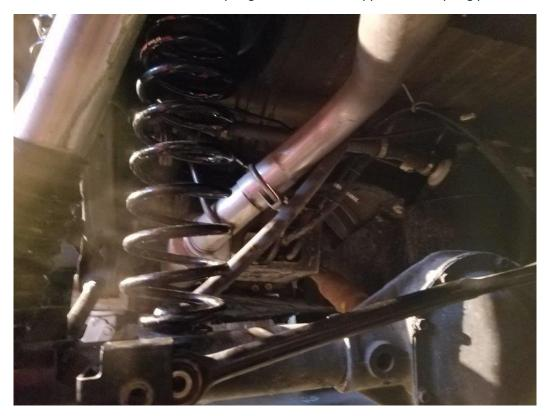
**12.** Now jack up the axle until the lower shock mount lines up with the bolt holes and reinstall the shock bolt. Torque to 65ft/lbs.
