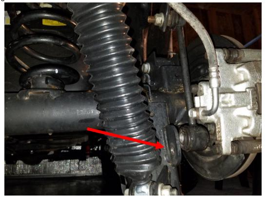
**3.** Using a 21mm socket, fully remove the axle side track bar bolt.
