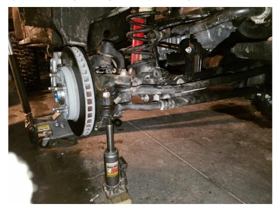
5. Remove the 18mm nut and bolt from the bottom of the shock. If the jack has relieved all the pressure the bolt will slide out easily. Also remove the 10mm bolt holding the brake line bracket.
