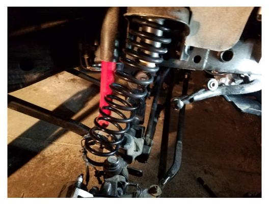
10. Now jack up the axle until the lower shock mount lines up with the bolt holes and reinstall the shock bolt. If you removed the brake line bracket you will want the brake line on the rear side of the shock as shown below. Using an 18mm socket and wrench torque to 72ft/lbs.
