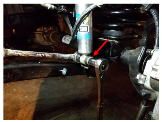
**11.** If you removed the brake line bracket, use tip ties to attach it to the shock. This will help keep them out of harm's way. I recommend using 4 zip ties. 2 are loosely placed around the brake line and abs wire (they are loose to allow the line to move side to side), 2 go around the shock and hold the 2 loose zip ties to the shock.
