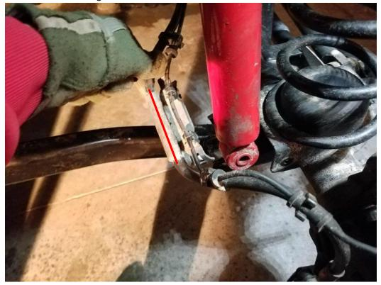
7. Now, using the jack under the axle, slowly lower it until the coil spring is loose. Then remove the spring. This will require the jack under the frame to be as high as possible. Keep an eye on the brake line and ABS wire, be careful not to overstretch them.
