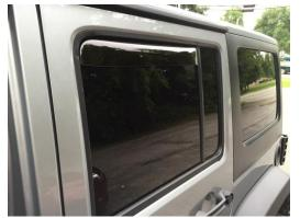
**Step Eleven:** Now proceed to put the window up and down carefully and slowly(Do this 5 times) to make sure the deflector flange is resting in the main window channel between the window glass and the rubber seal.
