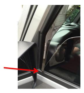
**Step Five:** Bow the deflector outward and insert the right edge of the deflector into the window channel as shown in the left picture below. Push the right side of the deflector up almost all the way leaving a ½" gap at the top right corner of windown as shown in the right picture below.
