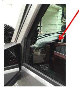
**Step Four:** Starting with the driver window first, place the left side of deflector on the top of the window sill like shown below.
