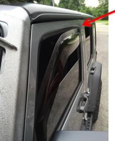
**Step Six:** Pull down and tuck the deflector in from left to right with the thin machined flange of the deflector fully and evenly inserted into the window channel.
