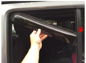
**Step Ten:** Push the deflector up into place like shown below with the thin machined flange of the deflector fully and evenly inserted into the window channel.
