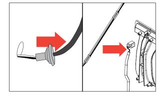
20. **Final Adjustment:** Tire bracket should be rotated and translated so as to move tire as close to main arm as possible.
