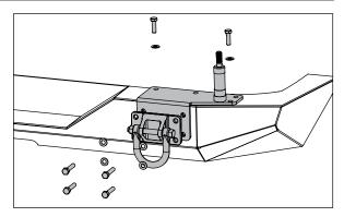
5. Install Bottom Spindle Cap onto spindle. Install bearing onto spindle. Ensure widest portion of bearing is on bottom.
