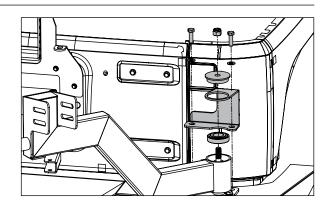
9. Install Tire Bracket to Arm using supplied short M12 hex bolts, M12 fender washers, and nylon lock nuts.
