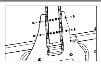
11. Assemble rod ends and jam nuts as shown.
