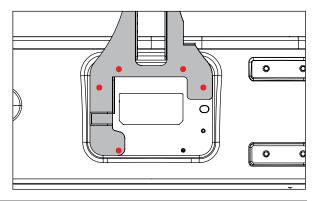
4. Remove right D-Ring from bumper. Install Spindle Bracket by inserting four hex bolts and washers supplied with rear bumper through Spindle Bracket and D-Ring. Thread two medium M12 bolts with washers into top of Spindle Bracket.
