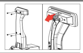
3. Remove existing tire carrier. Attach Tailgate Bracket to tailgate using factory hardware in locations shown in red.
