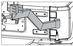
8. Install other bearing onto spindle, ensuring the widest portion of bearing is on top and will align with bearing surface of Arm. Install Spindle Brace over arm, followed by Spindle Cap and Castle nut. Fasten Spindle Brace to Spindle Bracket using supplied medium M12 hex bolts and washers.
