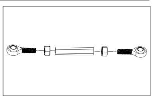
12. Install linkage, connecting main arm to tailgate bracket using supplied long M12 bolts, washers, nylon lock nuts and M12 spacers.
