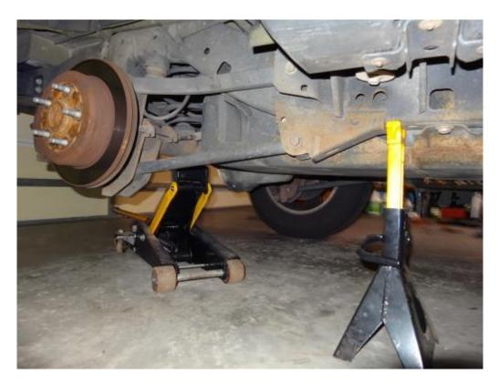
3. Disconnect the stabilizer bar link lower nut and bolt (18mm), lower shock nut and bolt (18mm) and brake line bracket bolt (10mm).
