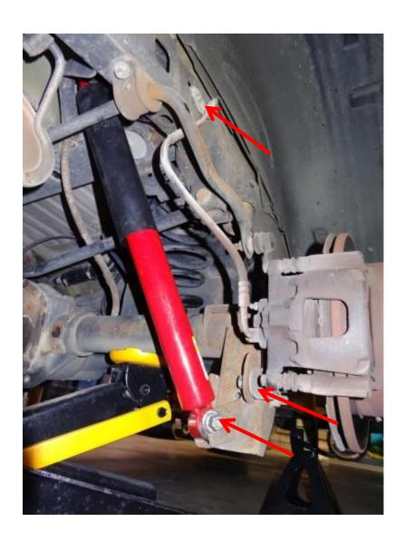
3. Lower jack to allow axel to drop and remove the rear spring and rubber isolator.
