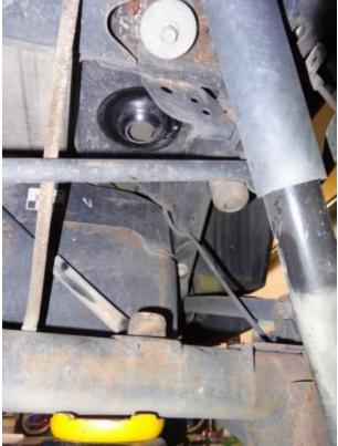
4. Position the 1 inch spacer on top of the rubber isolator and reinstall the spring.
