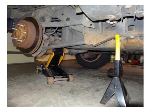
Raise the rear axle with jack and disconnect the stabilizer bar link lower nut and bolt (18mm), lower shock bolt (18mm) and brake line bracket (10mm).
