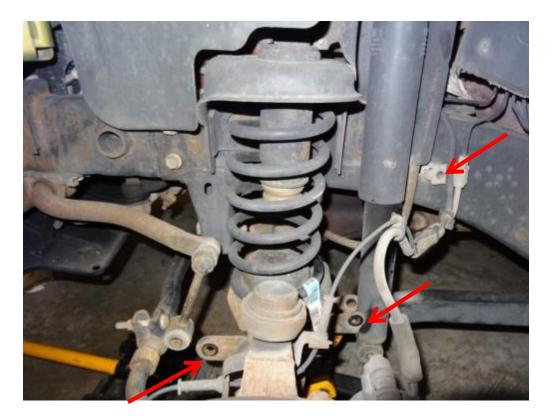
4. Lower jack to allow axel to drop and remove the front spring and rubber isolator.
