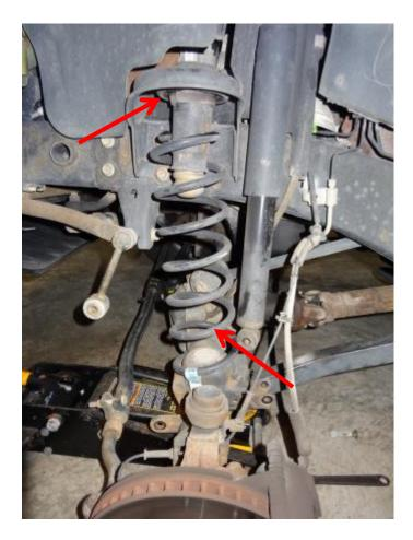
5. Position the 2 inch spacer on top of the rubber isolator and reinstall the spring.
