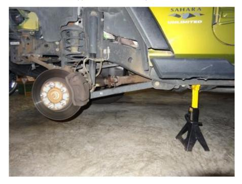
2. Use jack under the axel to lift axle.
