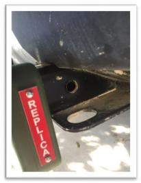
3. Install the hitch pin through the hole in the receiver and the hitch plug tube.
