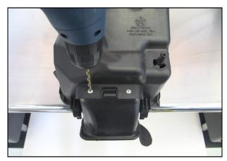
**4.** Drill out the rivet heads on the factory airbox and remove the air scoop. Remove any remaining rivet pieces from the air box and discard them.
