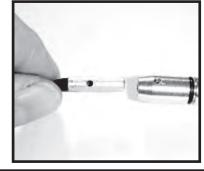
Step 3. Align the hole in the dipstick, sleeve and handle. Insert the pin removed from the factory handle using a small punch to set the pin.
