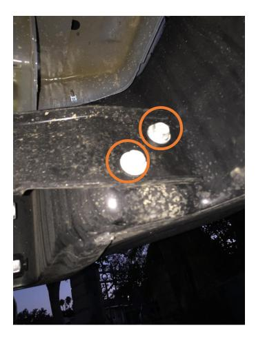
2. Once the 6 bolts are removed you will see the metal frame on the Wrangler where you will install the 4 bolts.
