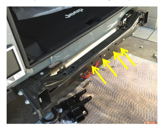
3. Install the four bolts by placing the flat washers in between and putting Loctite on the Nylock Nuts.
