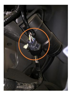
3. Take the trailer connector and run it through the taillight opening and down the foam insulator to the trailer hitch and slide into position.
