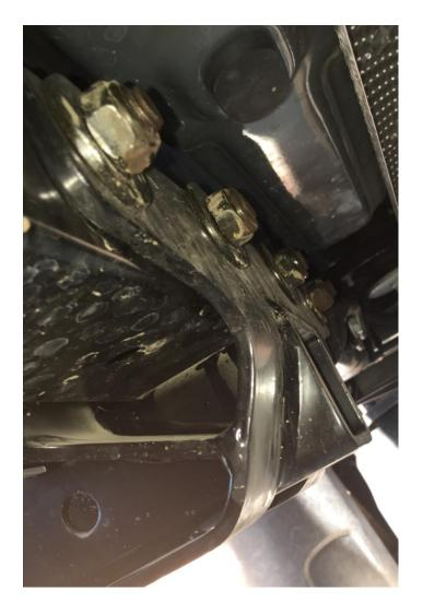
4. Install the bumper by installing the 6 bolts initially removed.
