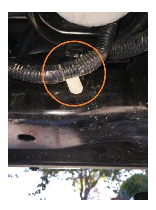
5. Place a spacer between the nut (with loctite) and the receiving end and tighten.
