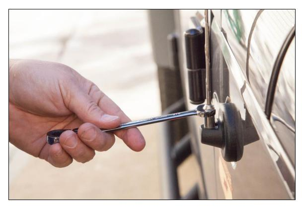
3. Unscrew the factory antenna by hand in a counter-clockwise direction until fully disengaged.
