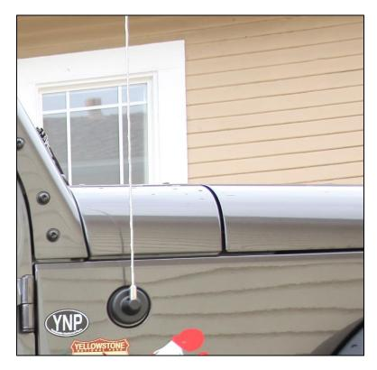
2. Loosen the factory antenna using a 3/8 inch open end box wrench or adjustable crescent wrench.
