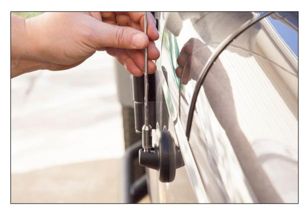
4. Attach the new RedRock 4x4 Trail 13 in. Short Antenna and tighten by hand until secure.
