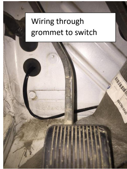
wiring from engine behind clutch pedal - leading to switch
