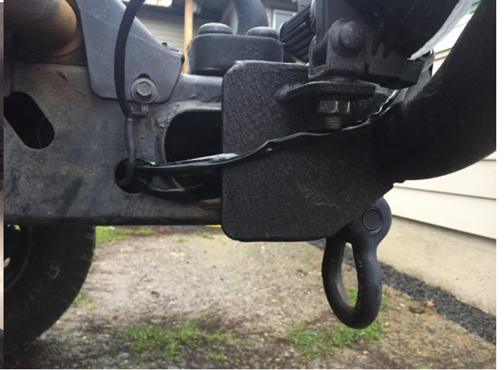
Wires leading through the bumper to the LED
