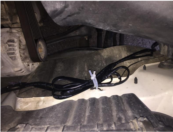
Wires leading from relay to LED (cleaned up)
