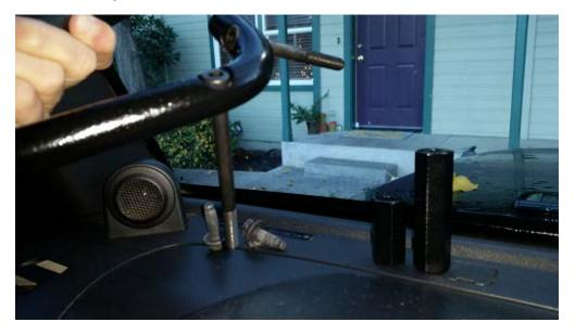
6. Install the upper bolt first, (ensuring the extension sleeve is already on the bolt), using the 6mm Hex socket. Only tighten enough to keep handle in place.
