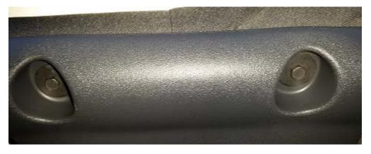
12. Install the handle using the 5mm hex socket with the wrench, tightening the two bolts by alternating between them until solidly in place (approximately 120lbs torque). Take care not to cross thread the bolts.
