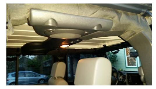
11. Remove these bolts using the 10mm socket with the socket wrench and extension.
