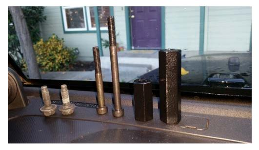
5. Push the bolts through the handle in the appropriate locations (short to top, long to side). Ensure you are using the correct handle for the correct side of the vehicle: the counter-sink holes should be towards the inside of the vehicle so the bolts can tighten down into them.
