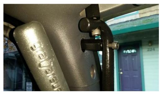
8. Alternate between the bolts, tightening until both cannot be turned further by hand (approximately 300lbs torque). Shake the handle occasionally to ensure there is no play while tightening, and be careful not to cross thread the bolts.
