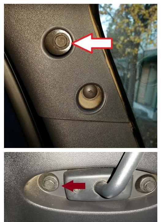
2. Use the paper towel under the bolt in the column to prevent losing the bolt inside the plastic housing. Remove the paper towel once the bolt is out.
