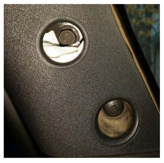
3. Remove the bolts located in Step 1, using the 13mm socket and wrench with extension.
