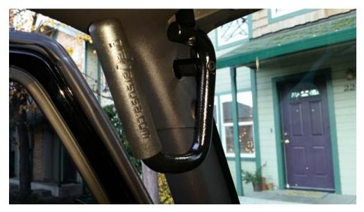
10. To install the Rear Handles, locate the bolts into the roll bar.
