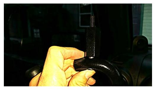
\*\*If you find this bolt having trouble threading easily, remove the handle and start the longer bolt into this upper hole without the handle. Once it is solidly in place, confirm the bolt is straight up and down. If it is not, the move the bolt by hand until it is (the nut in the upper part of the frame may not have been installed straight on, this will move it into place for an easier installation).\*\*
