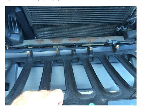
5. Next, you need to remove the **4 – T15 torx screws** that hold the ring securing the headlight in place.
