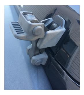
2. Once the hood is open you need to remove the **6 circular plastic fasteners** along the top of the grill. You can use a flat head screwdriver to pry them up but that might damage the lips of the
