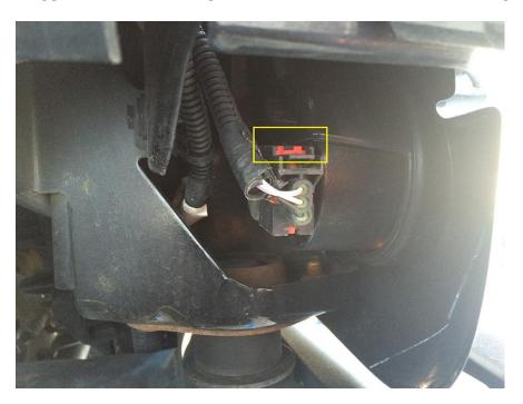
4. Once all 6 plastic fasteners are removed and the turn signals unplugged, you can start prying the grill off. The bottom of the grill has **4 clips** and there are **2 additional clips**, one on each turn signal. These clips just pop out.
