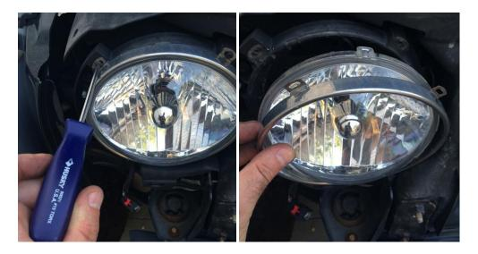
6. Once the ring is removed the headlight will fall out, make sure that you are holding it as you remove the last screw securing the ring. With the headlight out, unplug it by first clicking back on the red locking clip and then pushing down on the tab to remove the plug from the headlight.
