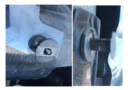
10. Once all 6 top fasteners are secure, plug the turn signals back in and secure the red locking tab, followed by closing and locking the hood. The install is now complete.
