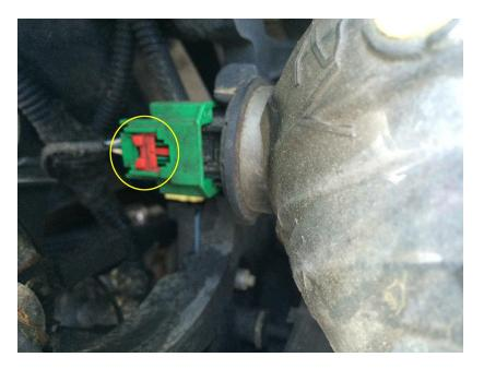
7. Next, plug your new light in and lock it with the red clip. These headlights came with an adapter harness that converts the wiring, so in this case the harness is plugged into the factory harness.
