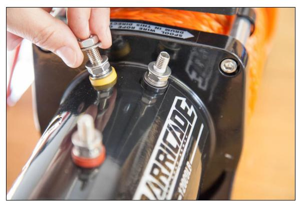
8. Shift the Control Box / Solenoid along the mounting bars to ensure the attached short, thick red, yellow, and black cables with connection rings will reach their respectively colored posts. Install cable connection rings over appropriately colored posts, ensuring raised portion of cable end is facing up.
