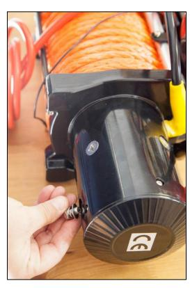
14. Locate loose black negative battery connection cable provided with winch. Install split washer and flat washer onto ground wire mounting bolt. Install connection ring from one end of loose black cable onto ground wire mounting bolt with raised cable end facing bolt head. Install thin black ground wire connection ring onto ground wire mounting bolt.
