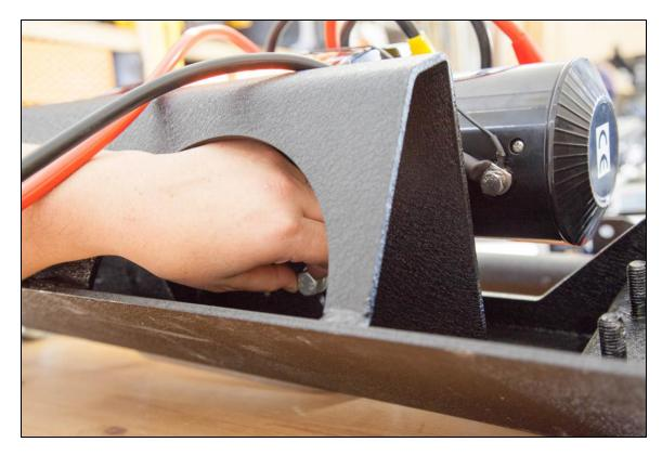
27. Tighten all mounting bolts using a 5/8 inch box, open end, or flex head ratcheting wrench.
