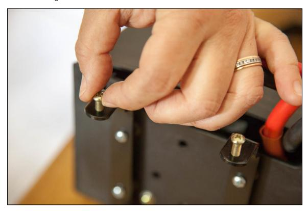
5. Position the rounded mounting arms of the Control Box / Solenoid against the front bar of the winch.
