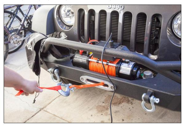
37. Install winch cover to protect synthetic rope from sun and weather, then hit the trails!
