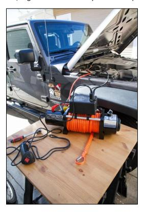
18. **OPTIONAL Part B:** Remove dust cover on winch Control Box / Solenoid receptacle and attach remote control cable. The receptacle and cable are keyed to help align the pins while connecting.
