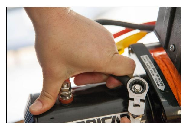
11. Slide the red, yellow, and black dust covers into place over the nut and post combos.
