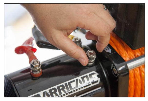
10. After short red, yellow, and black cables and hardware are in place, tighten each nut using a 14 mm socket and socket wrench or a 14 mm wrench.
