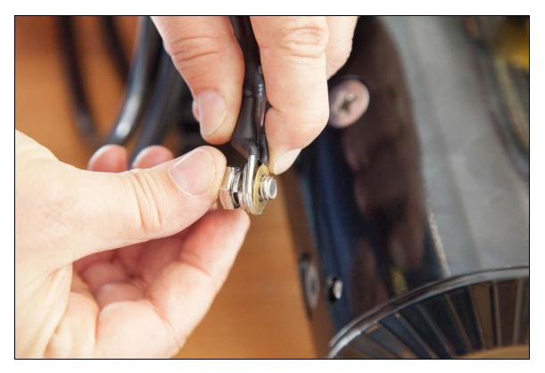
15. Reattach ground wire mounting bolt, hardware, and cable rings to winch mounting location and tighten using a 14 mm socket and socket wrench or 14 mm wrench.
