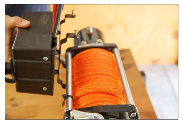
6. Lower the Control Box / Solenoid mounting arms onto the rear mounting bar of the winch so the cables connected to the Control Box / Solenoid are positioned at the rear of the winch. Do not tighten the interference bolts yet.
