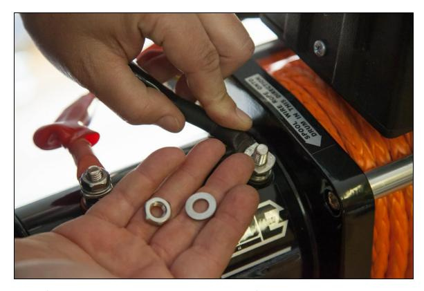
9. Reinstall one flat washer and one bolt onto each post and make finger tight.
