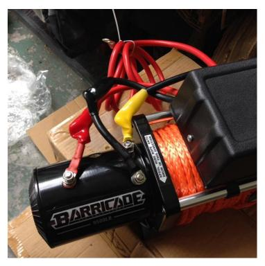
4. Roll the winch over onto its back side. Connect the black negative battery wire and black ground wire to the bolt on the underside of the winch using a 14mm socket. See picture below.
