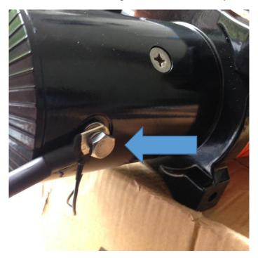
5. Return winch to the upright position. Place a bolt in opening of each of the four "legs" of the winch. See the below two photos.
