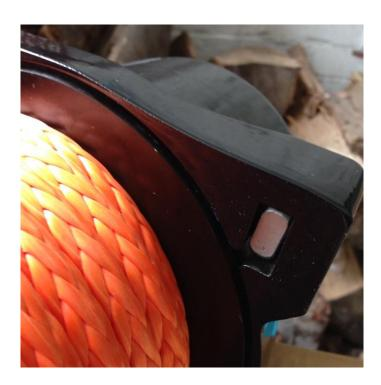
6. Place winch on bumper, being sure to line up the holes in the bottom of the winch with the holes in the winch plate. Install the winch with provided bolts and tighten with a 17 mm socket (a 5/8 socket also works). See the below picture.
