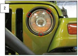
Remove the (3) T15 torx screws holding in the headlight bezel. Put these screws aside, they will be reused for the install of the guards.
