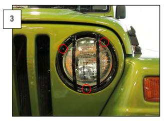
Place the headlight guard on top of the head light and secure it with the (3) T15 torx screws that were removed in step 2.
