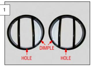
These guards are side specific. Lay both guards face up on a table. Position the center hole at the bottom with the dimple to the lower inside of the guard. This is how they will be installed on the vehicle.
