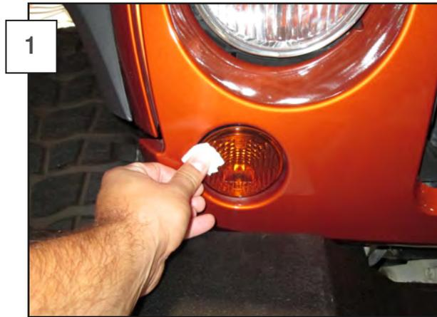
clean the turn signal guards with the supplied alcohol pad.
