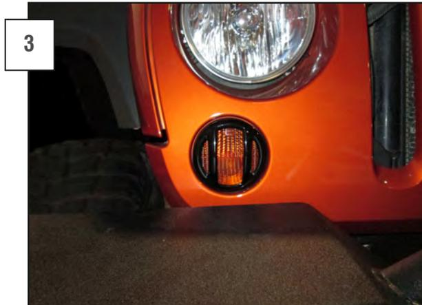
Lay the guard on top of the light and press around the edges to seat the 3M tape.
