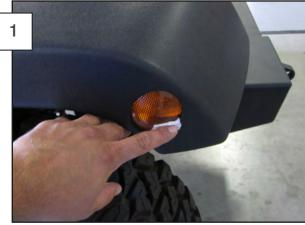
Clean off the marker lens with the supplied alcohol pad.
