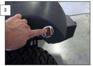
Install the marker guard onto the lens, then press along the edges of the guard to properly seat the tap around the circumference.
