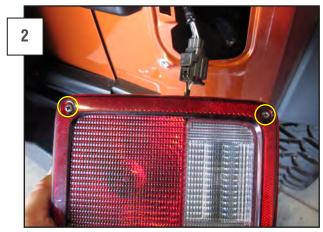
Remove the (2) outer phillips screws from the tail light lens. There will be a plastic trim piece behind the light that will become loose, be sure to secure it while removing the screws.
