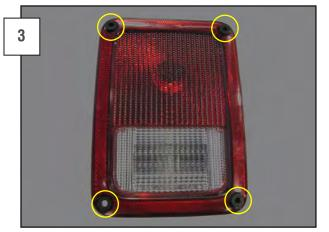
Hold the light face up and lay (4) of the included rubber screw buffers into the screw holes in the lens. Keep the lens facing upward until the guard is on.
