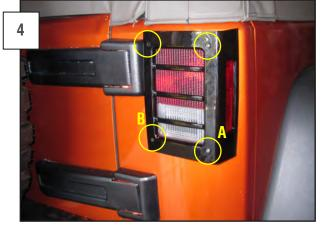
Place the guard over the light and (A) install the (2) outer phillips screws. This will hold the rubber screw buffers in place. Place the tail light back onto the vehicle and reinstall the (2) inner screws. Do not overtighten the screws.
