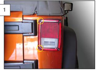
Remove the (2) inner phillips screws from the tail light lens. Keep these seperate, they are different from the outside (2) screws in step 2.
