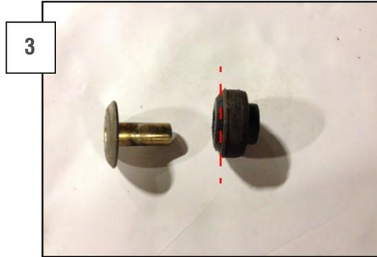
To allow for the thickness of the slider, the bushing needs to be cut down. Measure 5mm, or about .2in, from the top of the bushing and cut.
