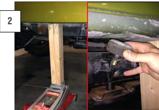
Jack up the body using a sturdy block of wood. (Pictured are two 2x4s screwed together) Using the raised body rail that rests on the body bushing, jack up the body slowly until you can remove the two rear bushings.
