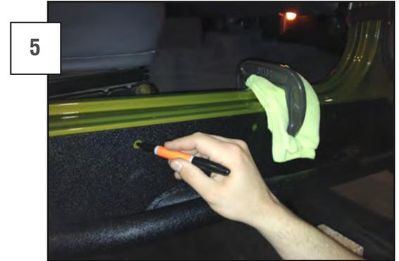
Use C-clamps on the front and rear of the slider to pull the top of the slider flush to the body. Mark and center punch each hole. Drill a pilot hole with a 1/8in bit, then follow it with a 3/8in bit. De-burr the edges of the holes, then use touch up paint or clear coat to prevent rusting.
