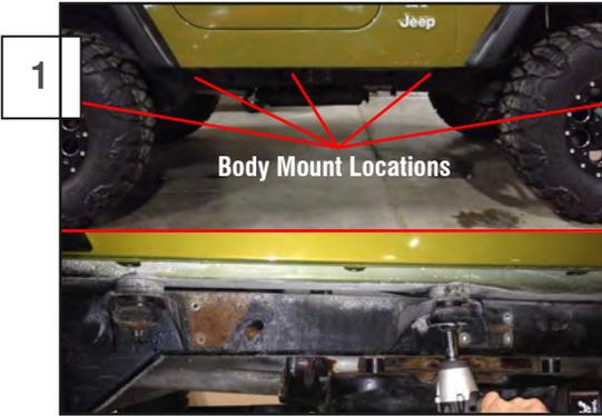
Begin by locating the five body mounts that run along the frame of the vehicle. There are three along the main frame rail and one on each front and rear bumper.
