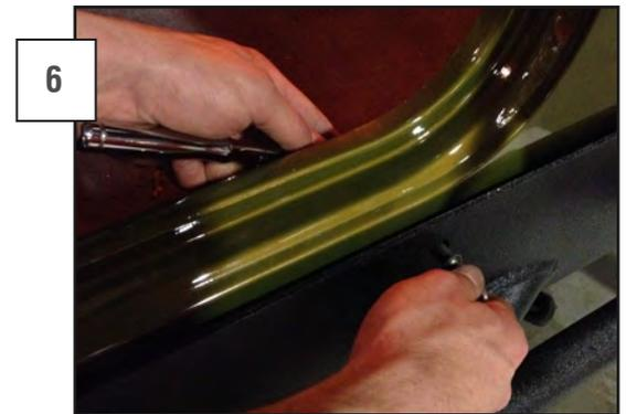
With the holes drilled and the slider secured by the body mount bolts, use the provided allen wrench install the bolts, with a washer and nut on the opposite side.
