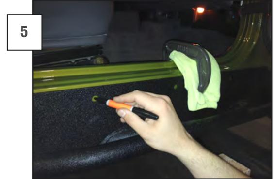
Use C-clamps on the front and rear of the slider to pull the top of the slider flush to the body. Mark and center punch each hole. Drill a pilot hole with a 1/8in bit, then follow it with a 3/8in bit. De-burr the edges of the holes, then use touch up paint or clear coat to prevent rusting.
