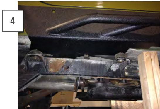
Once the rear two bushings are cut, replace them on the frame brackets, leaving about a 1/2in gap between the metal sleeve and rubber bushing. Lower the body enough to thread the bolt in a few turns by hand. Slide the slider between the metal sleeve and rubber bushing, making sure it sits flush against the body. When you are happy with the placement, slowly lower the body back onto the mounts.
