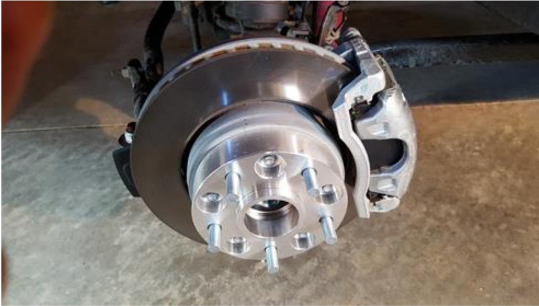
6. Using the included red loc-tite apply a small amount to the threads of the 5 nuts that came with the spacers.
