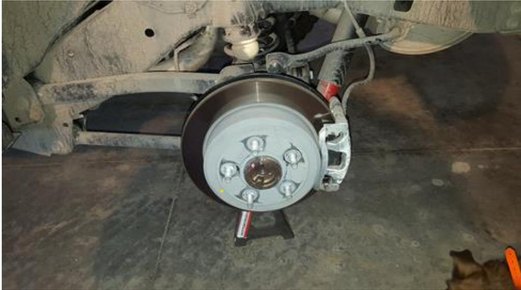
16. Following install it is very important that you check the wheel spacer nuts periodically to ensure they stay tight. You should check them after the first 100 miles, then at least every 3000 miles after that to be safe. When checking them I recommend you set your torque wrench to 95ft/lbs to ensure they are tight but not break the loc-tite seal if they are.
