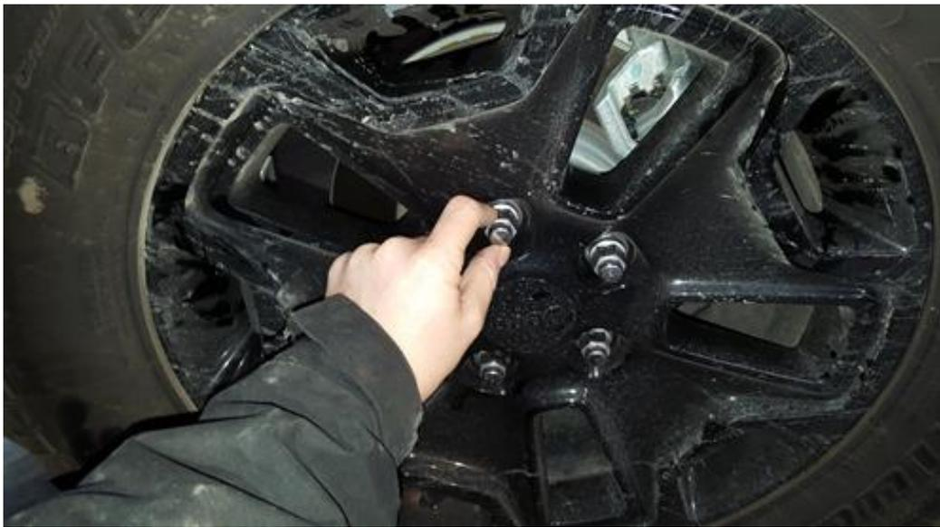
11. Now you can lower the wheel back to the ground. Then, using a torque wrench, 19mm socket, and extension, torque each lug nut to 100 ft/lbs using the same star pattern.
