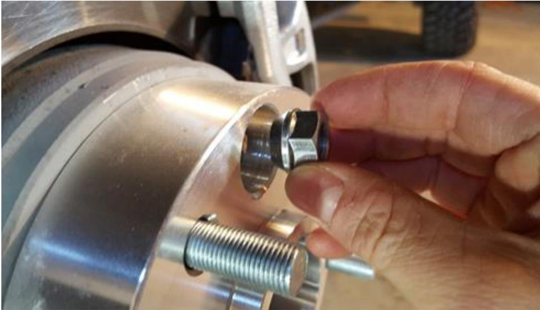
8. If you have a helper they can hold the brakes while you torque the nuts. If not, place a screwdriver in the rotor to hold it still while you tighten the nuts. First mildly tighten them in a star pattern as shown below. Then, using a torque wrench and 19mm socket, go back over each one and torque them all to 100 ft/lbs, again using a star pattern.
