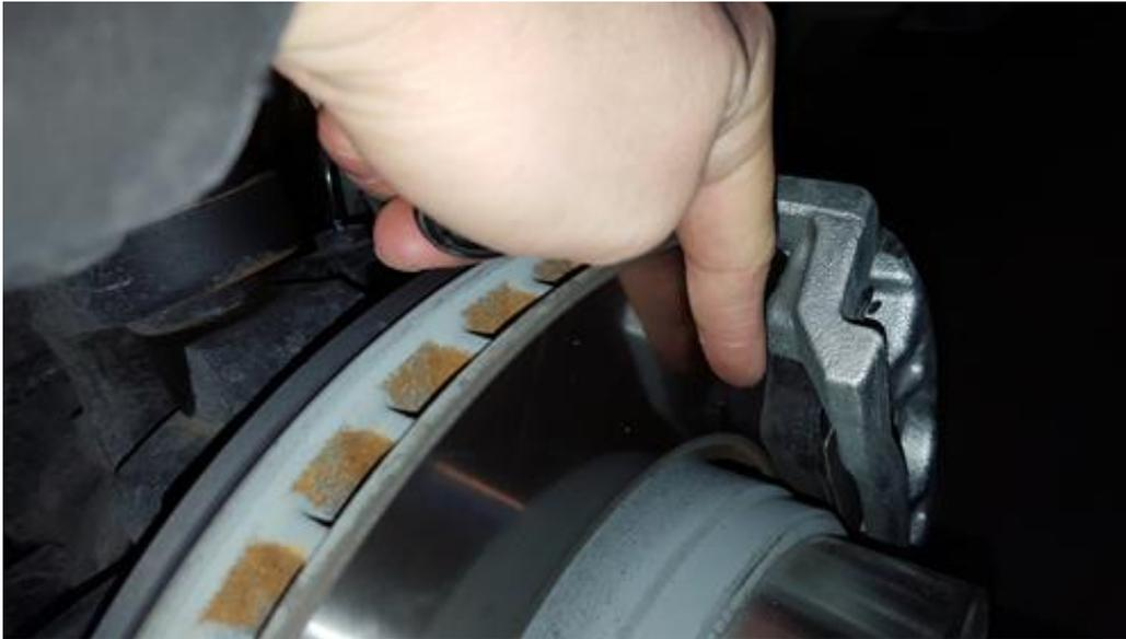
10. Now put your wheel back on and hand tighten all the lug nuts. You will want to push the tire up, down, left and right while gradually hand tightening all the nuts. Do this until they are all hand tight and the wheel won't move. Next mildly tighten the lug nuts in a star pattern.
