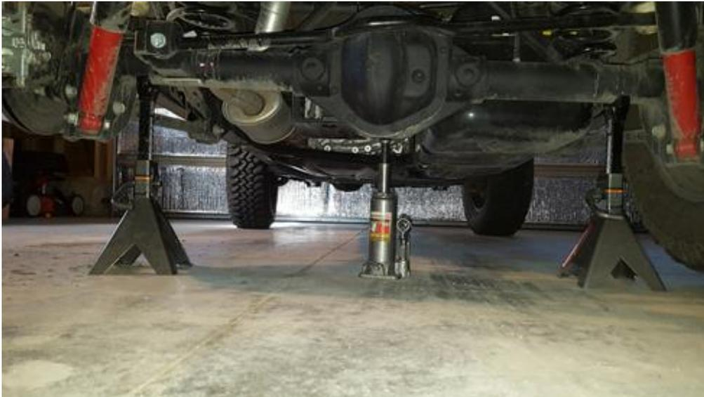
15. Install the rear spacers by repeating steps 4-11. There are only 2 minor differences when installing the rear. First there are 4 assembly washers to pry off instead of just 2. Next, when tightening the spacer nuts you can set the emergency brake and/or put the jeep in gear to keep the hub from spinning.
