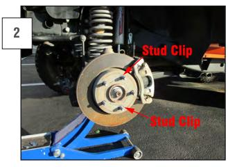
Remove any stud clips from the studs. They can be pryed up and clipped off. Care should be taken to keep from damaging the threads on the studs.
