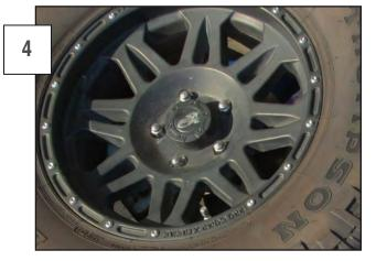
Replace the wheel onto the wheel spacer studs.
