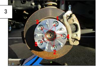
Place the wheel spacer onto the rotor, it will not fit flush against the rotor until the nuts are tight. Use the included wheel spacer nuts to secure the wheel spacer to the rotor. Tighten the wheel spacer nuts in a star pattern. Once they are hand tightened, use a torque wrench to torque each wheel spacer nut to 100 ft/lbs
