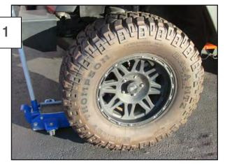
Loosen all (5) lug nuts a quarter turn. Raise the vehicle with a jack until the wheel and tire are off the ground. Brace the vehicle with a jack stand. Remove the lug nuts and remove the wheel from the vehicle.
