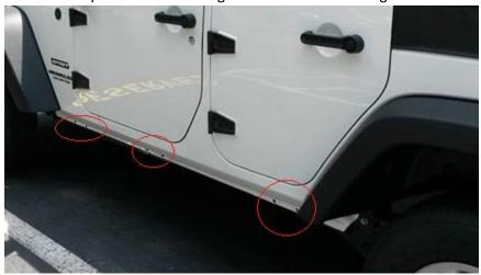
2. Insert threaded metal clip holes on underside of body. On 2015 JKU these clips may not be needed, as there is a threaded hole in place.
