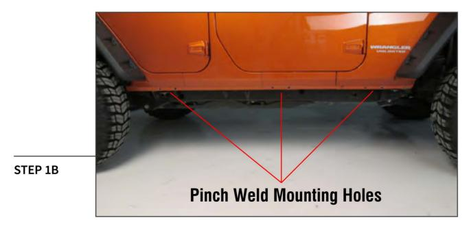
The metal clips are located directly behind each pair of pinch weld mounting holes. (4-door Wranglers only need (2) clips on the front and middle locations).
