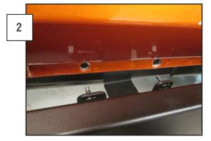
Before attempting to install, make sure you have the correct rail for each side. The front and middle mounting locations are offset towards the front of the rail/vehicle, this should help you figure out left and right.
