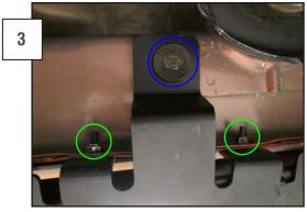
Once the rail is seated properly in each location, secure the pinchweld studs, marked in green, first with the supplied washers and lock nuts. Once the rail is aligned and secured along the pinchweld, install the supplied bolts, marked in blue. (2) botls per side for 2-doors, and (3) bolts per side for 4-doors.
