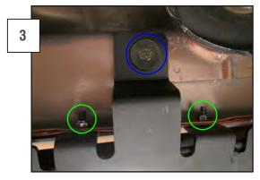
Once the rail is seated properly in each location, secure the pinchweld studs, marked in green, ÿrst with the supplied washers and lock nut s. Once the rail is aligned and secured along the pin chweld, in stall the supplied bolts, marked in b lue. (2) botls per side for 2-doors, and (3) bolts per side for 4-doors.
