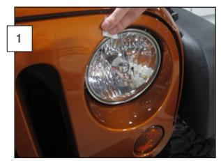
Using the supplied alcohol prep pads, thoroughly clean the area of the grille where the tape from the angry eye bezels will adhere.
