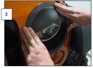
Once properly located, firmly press down on the outside edges of the bezel to fully seat the adhesive tape.
