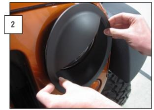
Peel the backing from the adhesive and place the bezel over the headlight opening as shown. Be sure to line up the bezel properly so it follows the contour of the grille.
