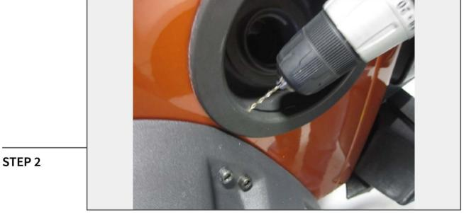
Remove the door from the vehicle and drill the four marked spots with a 7/64 bit as shown.
