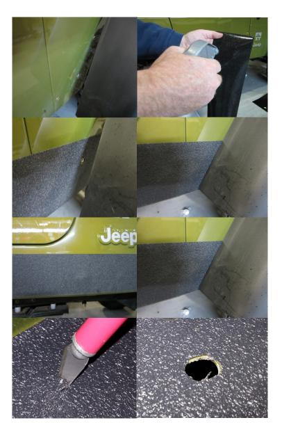
After installation you would do best by leaving ample dry time before driving or washing the vehicle, if you installed the recommended wet method. This is a permanent adhesive on this product. Great care should be taken if it is needed to be removed later.
