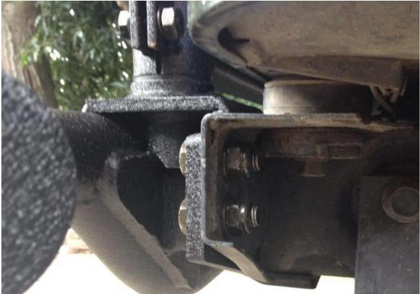
3. Install tire carrier by lifting it onto the tube with the zerc fitting. Should already come greased. First install nylon washer then install snap ring under the golden zerc fitting.
