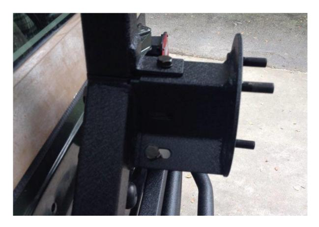
6. Install top post using a 24mm socket along with a crescent adjustable wrench or 24mm box end wrench.
