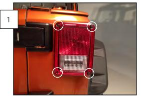
Support the light and remove the 4 stock phillips head screws from the tail light.
