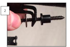
Place the plastic spacer between the light guard and the tail light. Use short screws on the inside of the light and long screws on the outside of the light. Be sure to use the washers on the screw heads.
