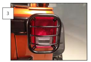
Install the light guard securely. DO NOT OVERTIGHTEN SCREWS.
