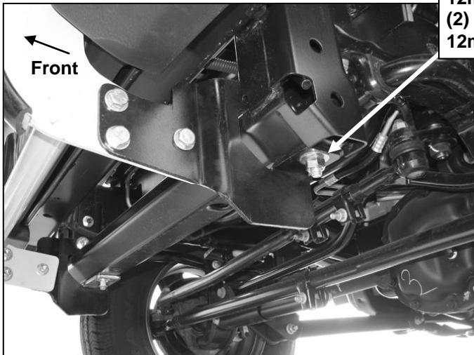
(Fig 15) All Driver/left side Frame Bracket installation
