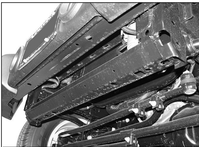
(Fig 1) Temporarily remove plastic splash guard
