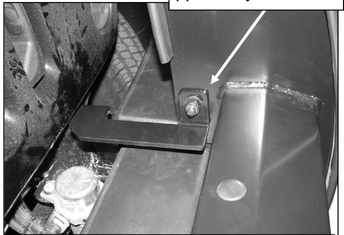
(Fig 16) All Driver/left side Top Bracket installation
