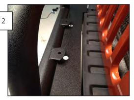
Lay the Filler Plate into place and align it with the stock, rear filler plate. The center holes are for routing wire. If lights are already installed, disconnect them and run the wires through the wire holes.
