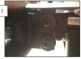
Reinstall the upper tube bumper bolt through the filler plate and tighten it down, while making sure the plate is level with the frame.
