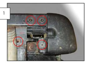
Remove the (3) T30 screws from the bottom of the bumper end cap. Also remove the (1) bumper to frame bolt above the exhaust pipe. Repeat on the opposite side. (For bumperette equipped vehicles, simply remove the bumperettes and continue to step 2.
