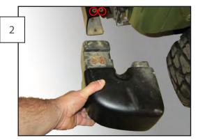
Remove the (2) T30 screws from the top of the bumper end cap. Remove the bumper end cap, by pulling it away from the bumper. Repeat on the opposite side.
