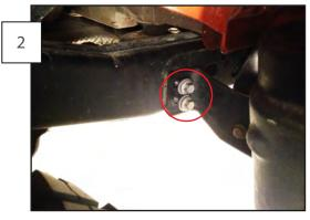
Remove the 4 stock 15mm stock bumper mounting bolts that are located on each side of the frame. Remove the bumper from the vehicle.
