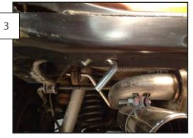
Insert the short side of the U bolt into, then out of the frame on the drivers side of the vehicle.
