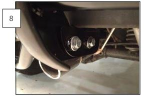
Hold the bumper guard in place and bolt it to the driver and passenger side brackets. Secure all hardware.
