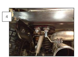
Attach the left side bracket to the u bolt. After reinstalling the stock bumper use the upper stock 15mm bolt to secure the top rear of the bracket.
