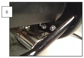
attach the right side of the bumper guard to the bracket and tighten all the hardware.
