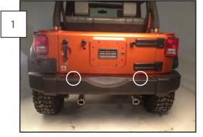
Remove the 2 upper stock 15mm, bumper bracket, bolts from underneath the vehicle.
