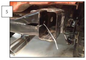
insert the bolt with extension wire welded to the head, through the frame, into the cross bar and drop it down into the existing hole in the frame.
