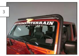
Start by mounting the vertical windshield mount first on one side, by installing the stock torx head bolts through the vertical support plate. Then install the horizontal bar. Keep all hardware loose at this point.
