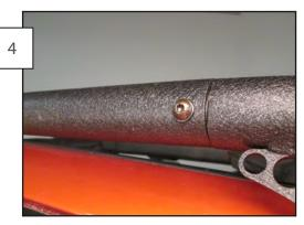
First slide the top of the bar into the horizontal section and loosely install the provided nut, bolt, and washers. Next, install the horizontal windshield bar. Double check that everything is aligned properly before tightening the rest of the hardware in place.
