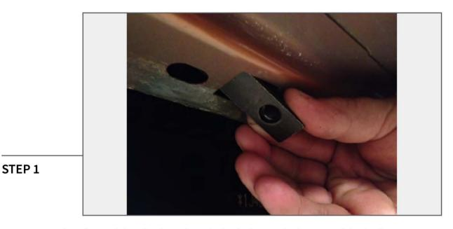
Insert a nut plate for each bracket into the existing holes on the bottom of the body.
