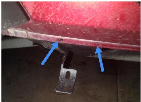
6. Secure bracket to side using 6mm allen head hardware (place small washer in the front (between nut head and Jeep pinch-weld) and large washer in the rear (between bracket and lock nut)).
