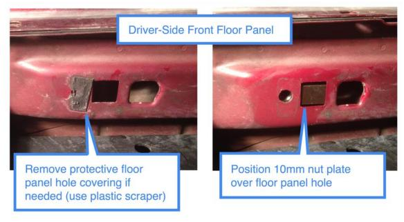
4. Hang the driver-side front (shorter) bracket by hand tightening the 10mm bolt (lock washer & flat washer) to the nut plate (or using the 8mm (x 28mm) bolts if installing on Jeep with factory threaded floor panels).
