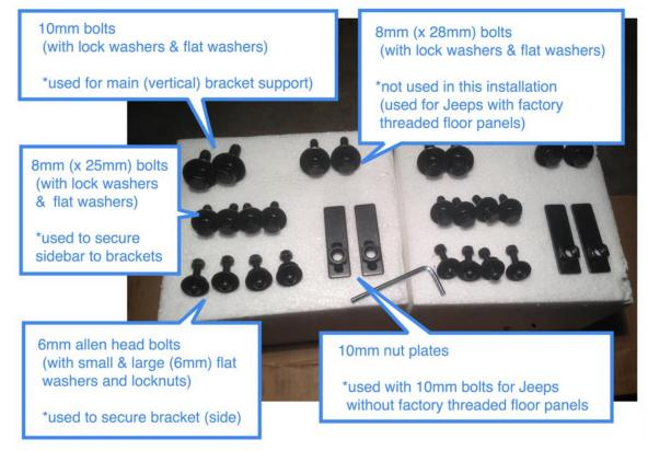
2. Identify passenger and driver-side front and rear brackets:
